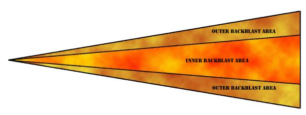
WHEN THESE WEAPONS ARE FIRED, THE POINT OF THE TRIANGLE IS PLACED AT THE REAR END OF THE LAUNCHER.
